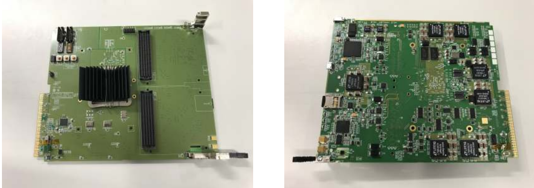
Figure 2: Front (left) and back (right) side of the FC7 with the Xilinx Kintex 7 FPGA and two LPCC FMC connectors.
