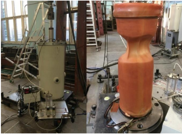
Fig 8 Picture of the triaxial test device and example of the sample at failure after the triaxial test with extension unloading [39].
