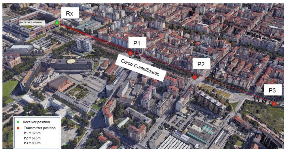
Figure 2. Setup 2. Transmitters (P1, P2 and P3) and receiver (Rx) position, with relative distance indications.
