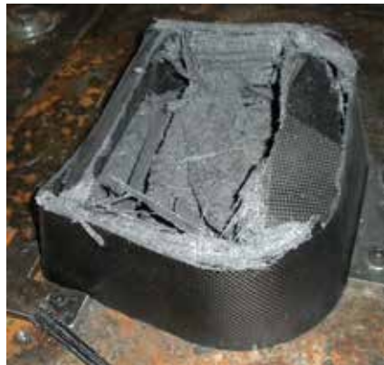
Figure 11: Full CFRP impact attenuator after the dynamic crush test.
