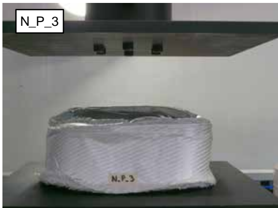
Figure 15: Full PURE ® impact attenuators before (left hand side) and after (right hand side) the crush test.
