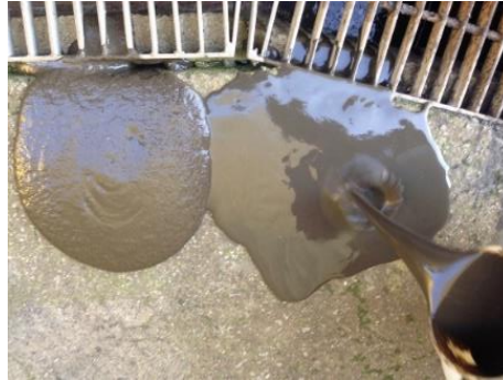
Figure 5. 11 Left un-treated WAS, Right treated WAS
