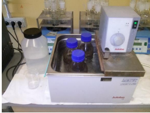
Figure 4. 1 Employed thermo-static batch reactor
