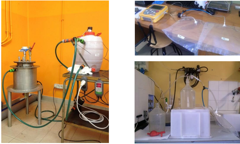
Figure 6. 1 - 12 L Anaerobic Reactor
