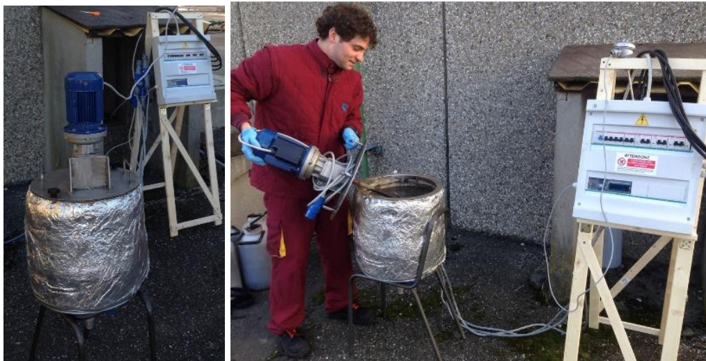
Figure 5. 1 Sludge pre-treatment. Employed Reactor and operation activity
