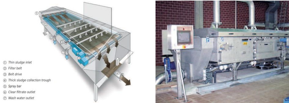
Figure 3. 2 Belt Thickener (Huber, s.d.)
