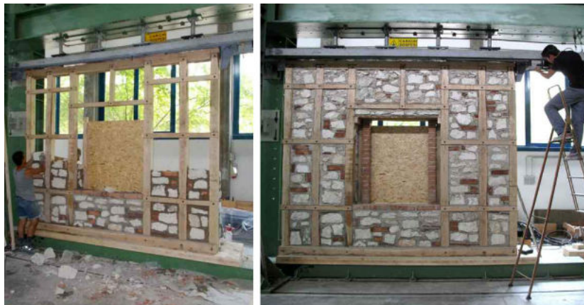
Fig. 4. Reconstruction of the “ Borbone ” seismic safety masonry building technology at the CNR-IVALSA laboratories.
