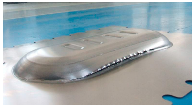
Fig. 4 Photograph of the deformed Ti6Al4V sheet
