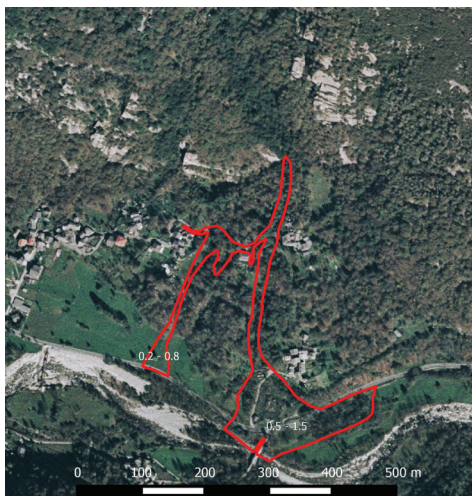
Fig. 8. Deposition area and debris thickness distribution of October 2000 Nora debris flow. [Colour online.]
