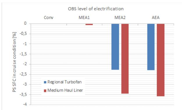
**Fig. 10. Influence of OBS electrification on engine SFC.**
