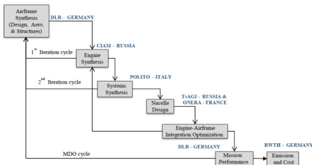
Fig. 1. MDAO workflow developed within AGILE research project.
