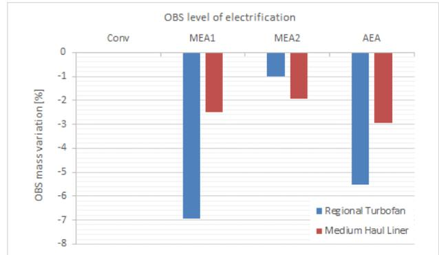
**Fig. 9. Effect of OBS electrification on systems mass.**
