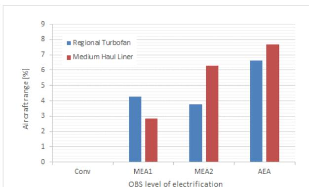
**Fig. 11. Influence of OBS electrification on aircraft range.**
