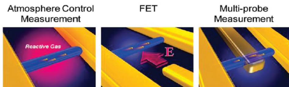
Figure 8. Schematic illustration of the strategy for investigating resistive switching mechanism in core-shell NWs by means of atmosphere-controlled measurements, field effect measurements in NW-FET configuration and multi-probe measurements. Adapted with permission. [197] Copyright 2011, American Chemical Society.
