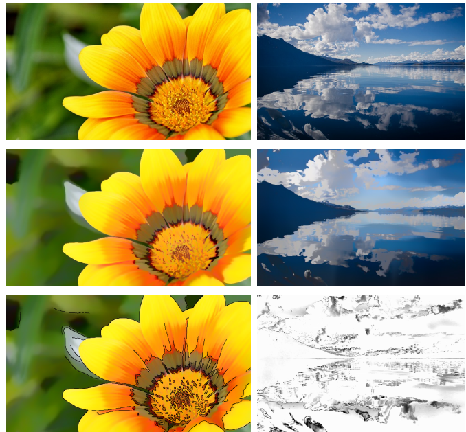
Fig. 10. Examples of non-photorealistic rendering. Image stylization is shown in the left column and pencil drawing is shown in the right column. From top to bottom: Original, edge-preserving smoothing, and NPR results, respectively. The method in [153] is used for edge-preserving smoothing. For stylization, the edge image is combined with the smoothed image. For pencil drawing, edge detection is performed to the smoothed image and the edge image is combined with the high-frequency information in the image. Both test images are obtained from https://pixabay.com/ .
