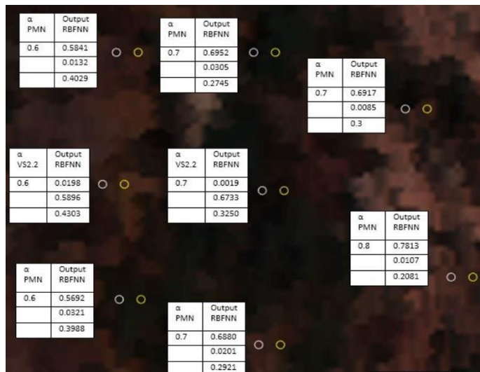
Fig. 6 : A sample of the output of the RBF when applied on one image. White circles represents the location of the inserted PMN mines in the image, yellow circles are the placement of the VS-2.2 mine.
