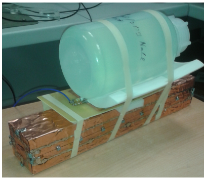
Figure 11. Measurement setup used to evaluate the effect of the shield on EPI images. All the images of the cassettes with the solid and the slitted shields were acquired at 4T.
