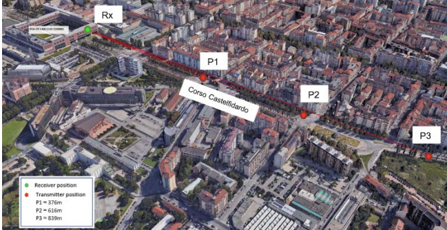
Fig. 3. Positions of the transmitter (P1, P2 and P3) and of the receiver (Rx), with relative distances for the point-to-point measurements.
