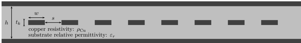
Fig. 6 Cross-section of the eight-conductor stripline interconnect. The deterministic values of the geometrical and material parameters are [15]: w = 0.127 mm, s = 0.127 mm, h = 0.508 mm, t_k = 15.24 \mu m, \rho_{Cu} = 17.241 n \Omega \cdot m, \epsilon_r = 4 .
