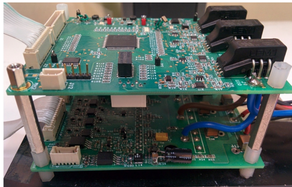
Fig. 3.44 Converter module: Low level control board and power board.
