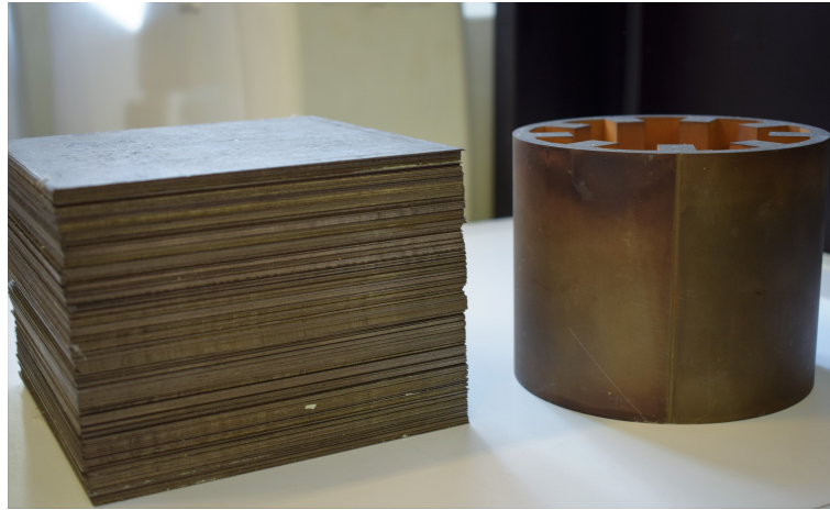
Fig. B.2 Pre glued iron block M250-35A and the stator obtained by EDM
