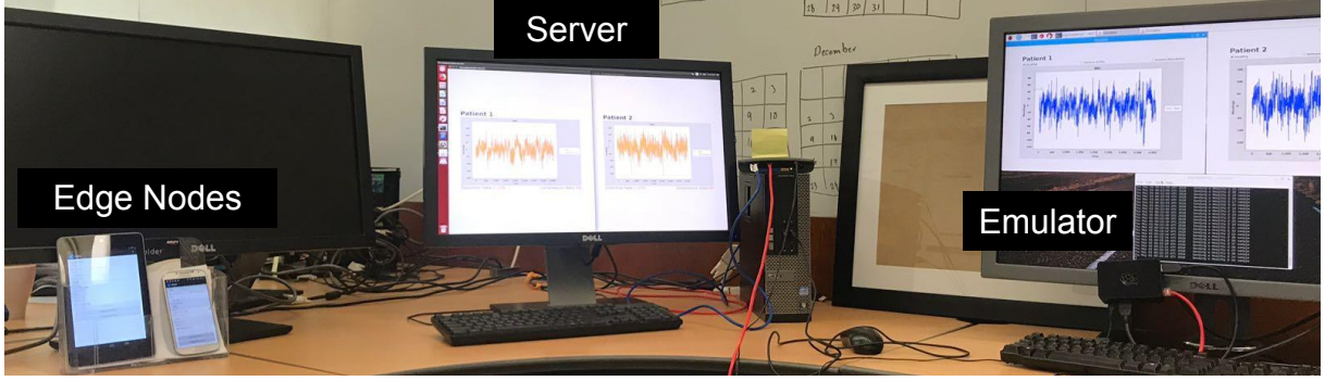
Fig. 9. The implemented system for EEG telemonitoring.
