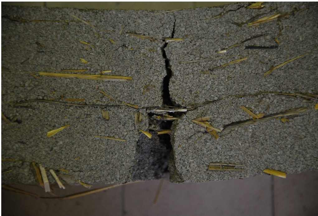
Fig. 5. Details of bending collapse of P series (straw fibers reinforcement)
