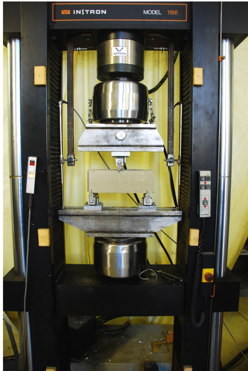
Fig. 3. Three points bending test through INSTRON MODEL 1186
