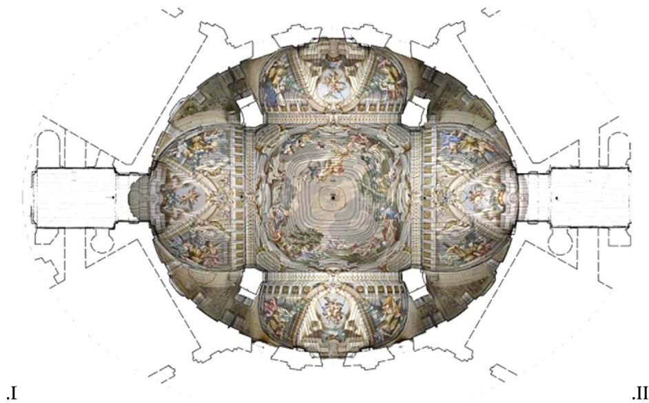
Fig. 5. Orthophoto produced by means of the SfM approach4 integrated in a 2D representation with contours (II).
