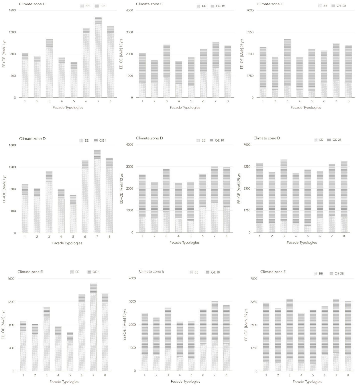
Fig. 5. Sum of EE (light grey bars) and OE (dark grey bars), for the 8 analyzed façade system typologies, with reference to three periods of time: 1 (first column), 10 (second column) and 25 years (third column). The graphs refer to the different climate zones. From above: London; New York; Chicago.
