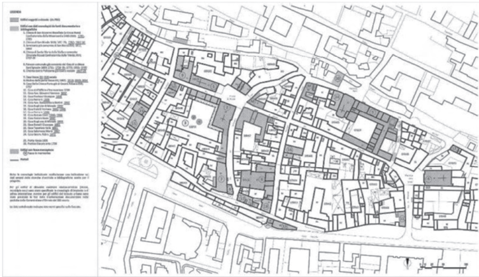
Fig. 3 The thematic table brings together and summarises the chronological data that emerged from the study of new sources in the archive research and from the material analysis of the buildings with a critical survey of the historical phases that changed the original plan. Piano di manutenzione of the façade surfaces of Saluzzo old town. Indicazioni di cronologia storica degli edifici . Plan - Table no. 7.
