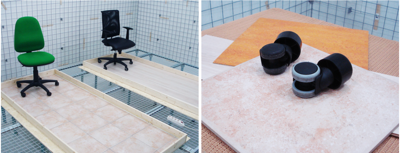
Figure 1. The materials tested in this experiment. In the picture on the left, the LLC and the HLC and two of the three paved platforms, provided with the wooden flooring and the ceramic flooring, placed on the floating grid. In the picture on the right, the LLC and HLC wheels provided with handles and one piece of each type of flooring.
