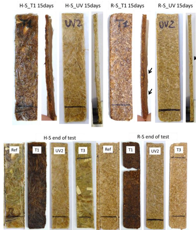
Figure 8. Digital pictures of pristine (Ref) and aged samples after 15 days and at the end of ageing tests.
