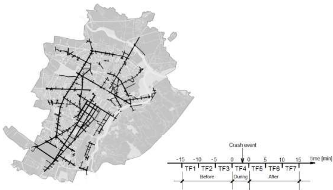
Figure 1. Turin's traffic monitoring network operated by 5T in 2006 (highlighted in black), and time scale used to aggregate traffic flows (TF) in the seven 5-minutes periods across the crash event.
