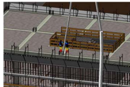
Fig 3. Modeling of the construction phase "casting with bucket"
