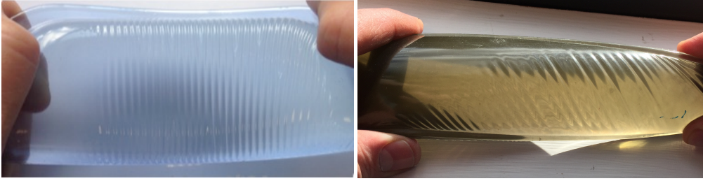
Figure 6: Formation of regular sinusoidal wrinkles on wrist supports made of gels enclosed by a stiff film casing, by bending (left) or torsion (right).
