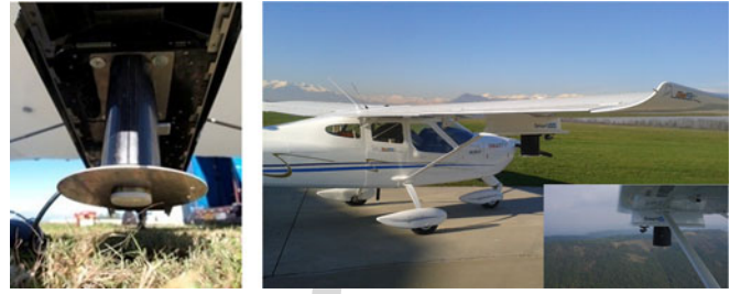
Fig. 3. GNSS-R prototype mounted on digisky P92 aircraft.
