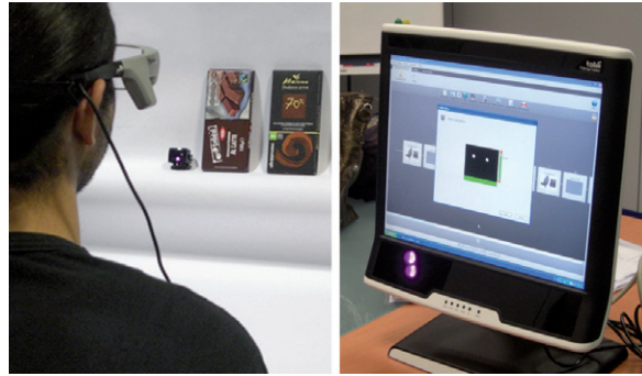
▲ Image 13. Eye-tracking device during tests carried out in MATto, Politecnico di Torino. Credits by the paper authors.
