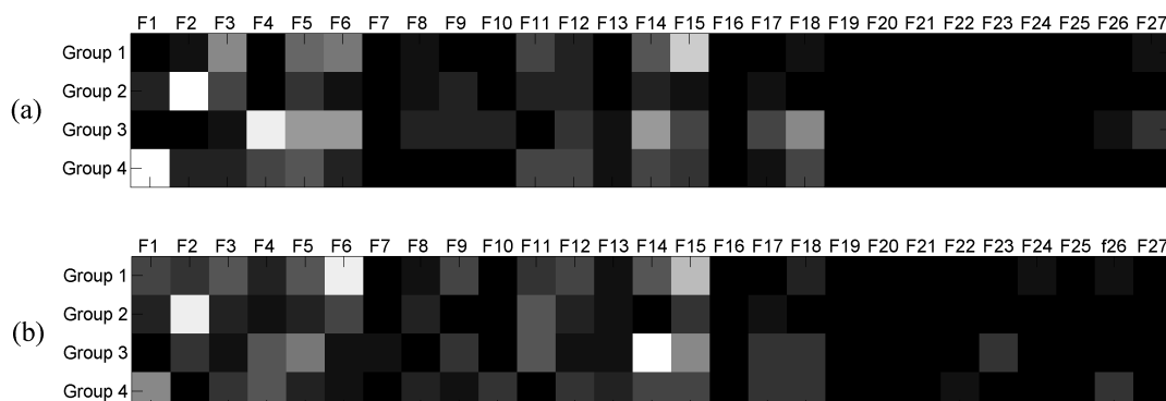
Figure 6.5: Results of the clustering algorithm applied to TF distribution of the COP signals recorded in (a) OE condition and (b) CE condition. Each row shows a group, each column shows a feature. Each cell displaces the number of times in which the feature is present in the group, normalized on the number of element of the group. There are 16 gray levels.
