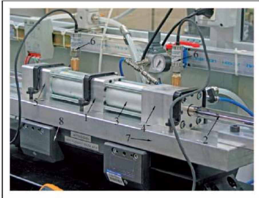
Figure 7: Rod seal friction measurement fixture
