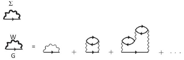
Fig. 2. The self-energy in a generally accepted approximation is represented by a propagator G multiplied by the interaction W and integrated over internal exchanged momentum. The effect of potential screening can be visualized as a summation over infinite ladder contributions.
