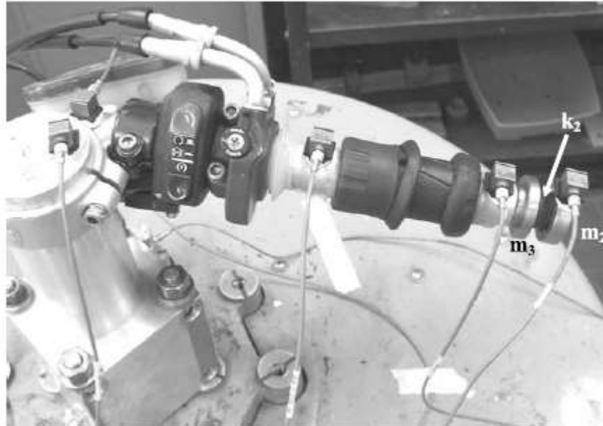
Fig. 9 The handle with the proposed vibration absorber
