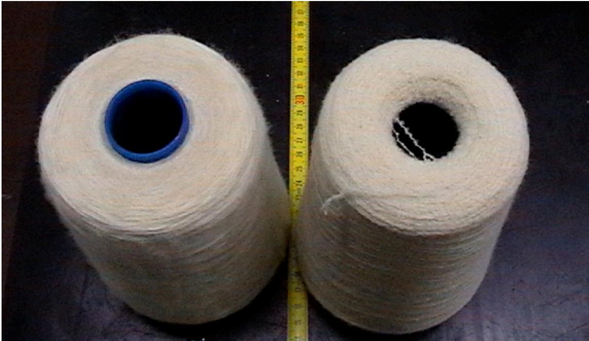
Figure 13 Bobbin obtained with metal opposite circular bases, left, without metal bases, right, after thermal cycle.
